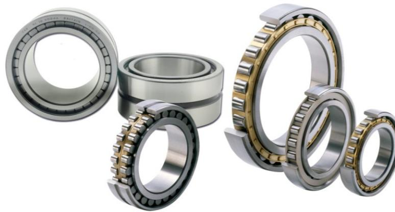
NPB cylindrical roller bearings are available in many designs, series and sizes. The majorities are single row bearings with a cage, single and double row full complement bearing. Bearings with a cage can accommodate heavy radial loads, rapid accelerations and high speeds. Full complement bearings incorporate a maximum number of rollers and are therefore suitable for very heavy radial loads at moderate speeds.
